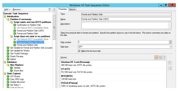
Figure 4-4: Format And Partition Disk task sequence step in a Create New MDT task sequence
