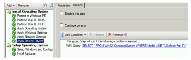
Figure 3-4: Condition set on a step via the options tab
