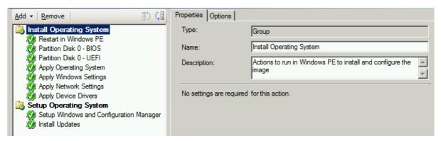
Figure 3-3: Default task sequence (created via the New Task Sequence Wizard) containing action steps
