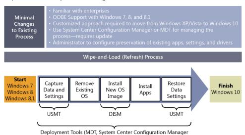
Figure 4-10: An overview of the wipe-and-load process
