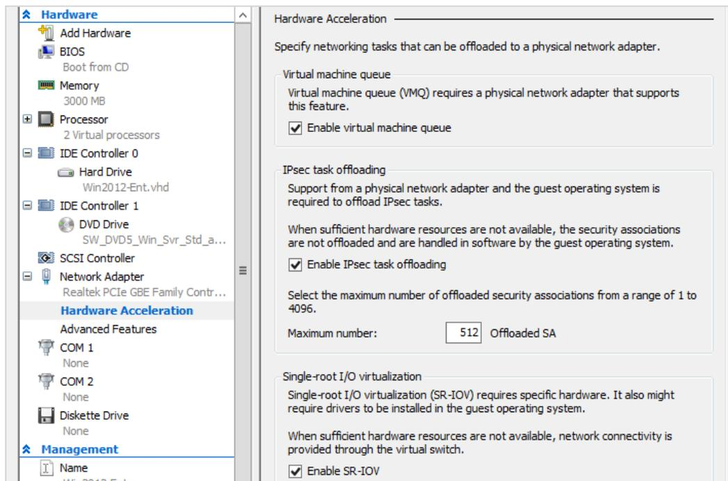
Figure 36 shows how SR-IOV attaches a physical NIC to a SQL Server virtual machine, which helps with the live migration of the virtual machine. In this process:
