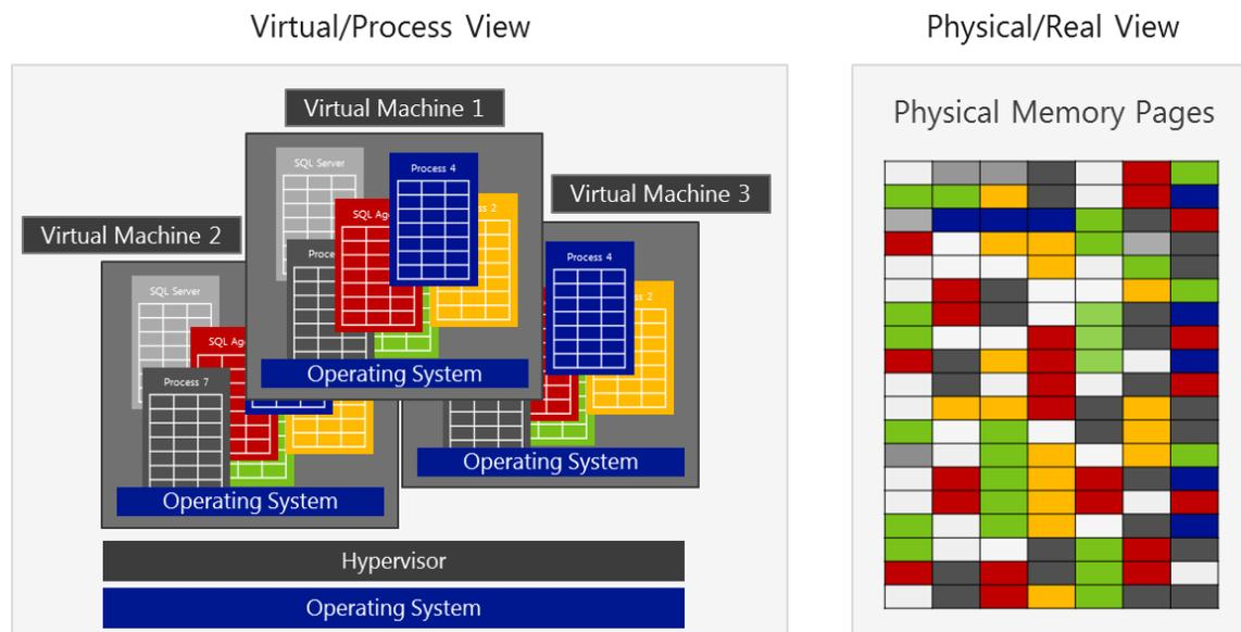
SLAT technologies also help to reduce CPU and memory overhead, thereby allowing more virtual machines to be run concurrently on a single Hyper-V machine. The Intel SLAT technology is known as *Extended Page Tables (EPT)*; the AMD SLAT technology is known as *Rapid Virtualization Indexing (RVI)*, formerly *Nested Paging Tables (NPT)*.
