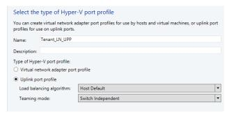
**FIGURE 3-13** Load balancing algorithm and teaming mode configuration for the Tenant\_LN\_UPP Hyper-V port profile
