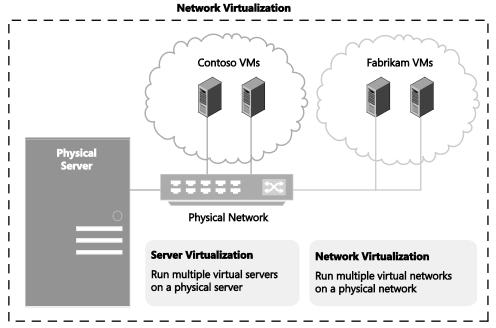
FIGURE 1-8 Logical architecture for network virtualization
