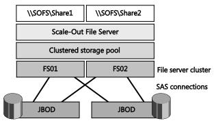
FIGURE 4-1 Logical diagram of a Scale-Out File Server
