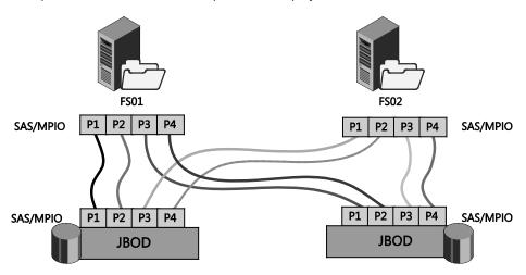
FIGURE 4-2 Two servers, each with two SAS HBAs in failover cluster configuration with two JBODs and **MPIO**
