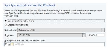
**FIGURE 3-11** Network site, IP subnet, and VLAN configuration for the Datacenter\_LN\_Pool1 IP pool
