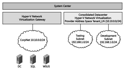
FIGURE 6-24 A representation of network virtualization configured with NAT and multiple, isolated VM networks
